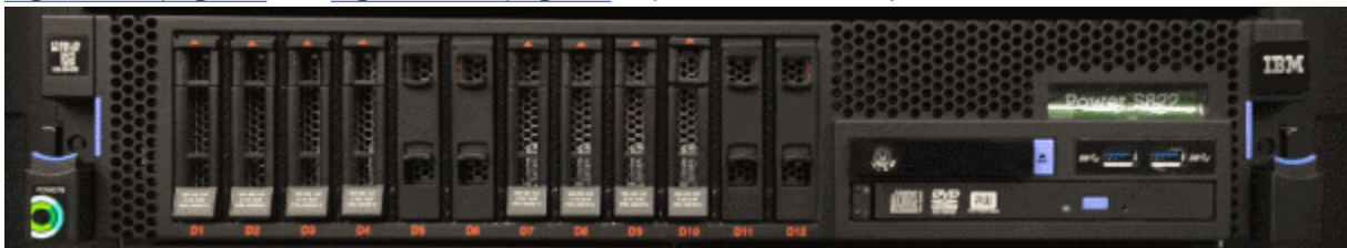
Figure 9. TS7760 Server (3957-VEC) System Unit (front view)
